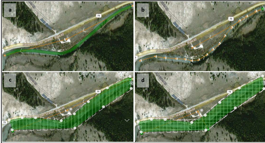
Figure 4. Four flight path types. (a) Linear flight path. (b) Waypoint flight path. (c) Grid flight path. (d) Cross-grid flight path. Flight path location is on the Salmon River just north of Lower Stanley, Idaho. Flight paths were designed using Yuneec's DataPilotPlanner (version 2.1.22).
