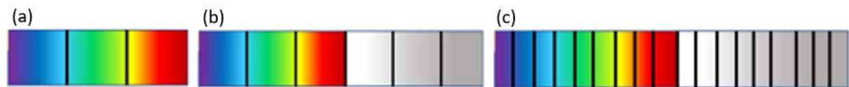
Figure 3. Three examples of sensor spectra: (a) RGB. (b) Multispectral. (c) Hyperspectral.
